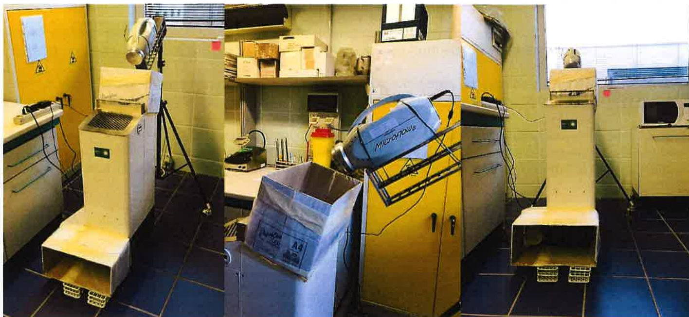
Figure 3. Setting around the device: the microbiological air samplers were placed next the inlet grid and on the outgoing air stream.
